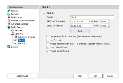
• In the **Slot #1** (or **Slot #2**) pane, specify the following slot-related parameters:
