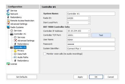
In the Controller pane, specify the following XRT Controller-related parameters:
