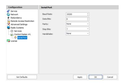
• In the **Serial Port** pane, specify the same serial port settings as those on the radio device connected to the serial port.
