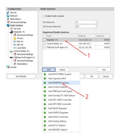
All radio system elements based on MOTOTRBO services are represented in the **Registered Radio Systems** table, including their type (Control Station, Repeater, and others), IP Address, and Radio ID (1):
