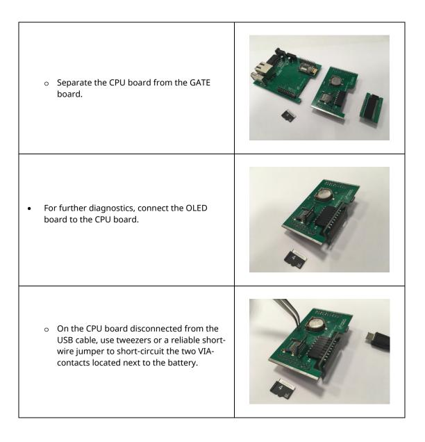
While keeping the contacts short-circuited, connect the CPU board via a USB cable to your PC with the installed Swift CPS.
