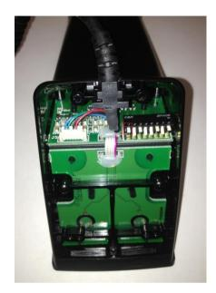
Remove the 5 screws on the bottom panel of the microphone. Remove the panel.
