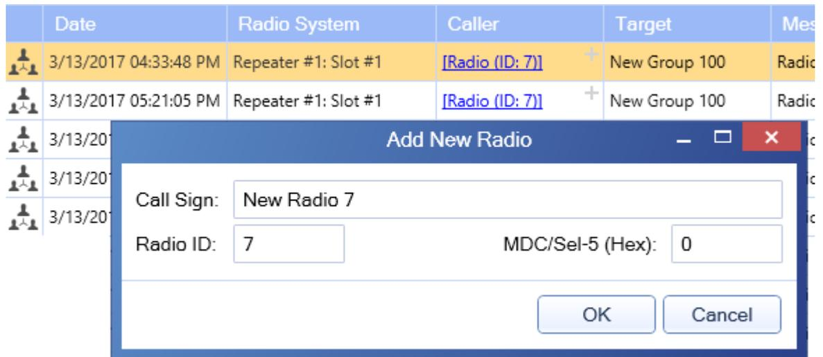
Figure 24: Registering an unknown calling radio
